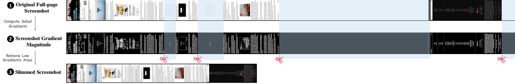
Figure 2: Illustration of the Screenshot Slim Process. We leverage Sobel gradients (Kanopoulos et al., 1988) to identify blank areas and remove them. After slimming, the screenshot size is largely reduced without any information loss.
