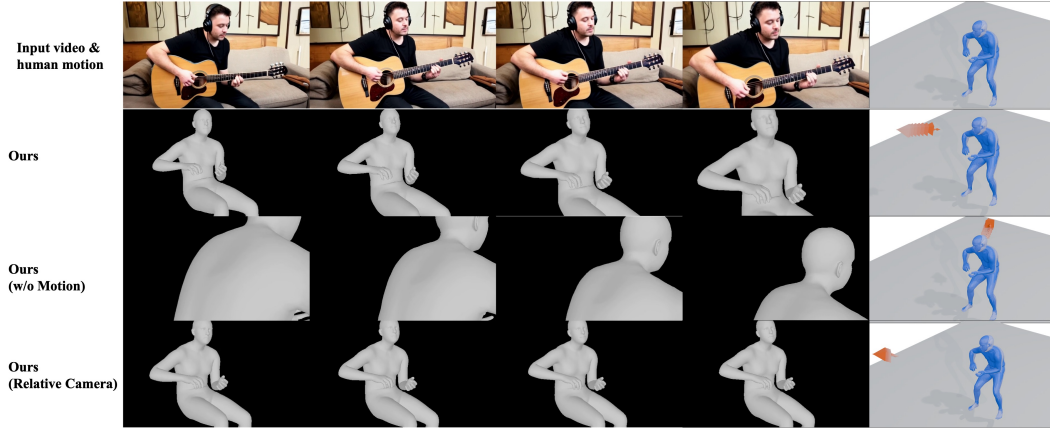
Figure 6: Columns 1–4 show the reprojection of 4D human skeletons by using estimated camera parameters, while Column 5 presents the rendered results in 3D space. w/o Motion exhibits viewpoint errors, whereas Relative Cam suffers from scale perception issues.
